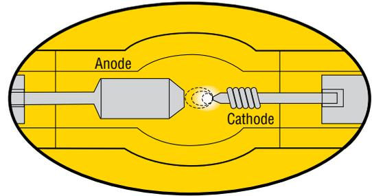
The construction of EmArc arc tubes, electrodes and precise filling technique provide the environment for the tightly confined plasma arc discharge. EmArc light output over time exceeds that of typical DC Xenon and AC short-arc Metal Halide lamps.
